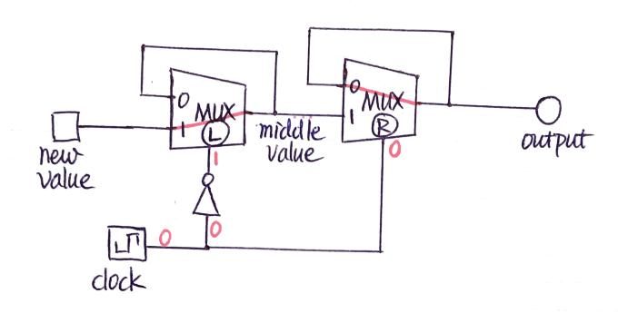
When clock = 0, MUX D is open. middle value = new value. MUX B is closed.
