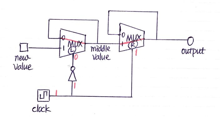
When clock = 1, MUX @ is closed. MUX @ is open. output = middle value.
